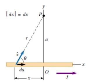
According to the Biot–Savart law, the magnetic field at point P due to element ds is given by
